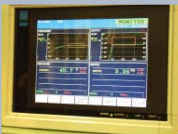
260 Process Monitor showing pressure and position curves.
