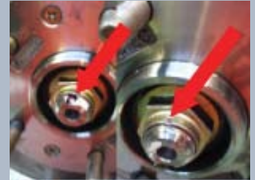
X Two Nuts Staked Incorrectly. Not in the slot
