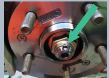
✓ Nut Staked Correctly. In the centre of the slot.
