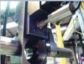
Staking Tool showing the Position Transducer measuring the Stake Depth
